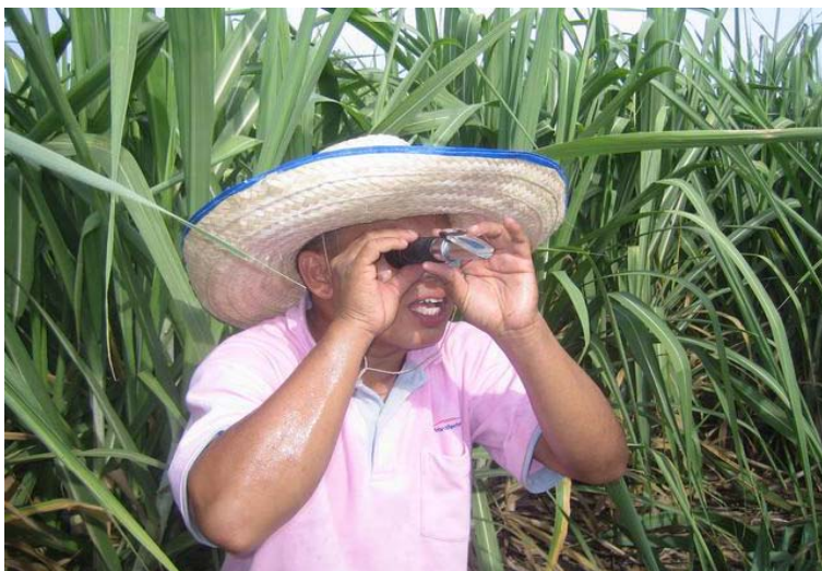
Brix testing inside of Sugarcane field
