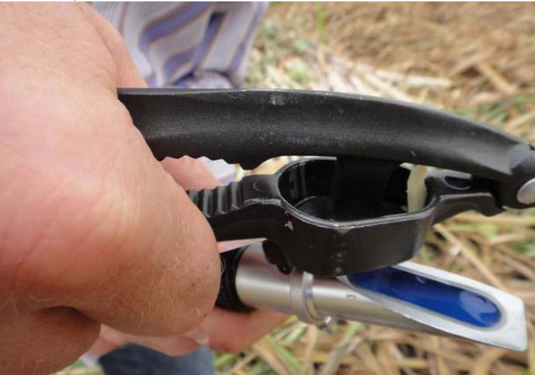
Pressing of cane-juice on to Brix-meter
