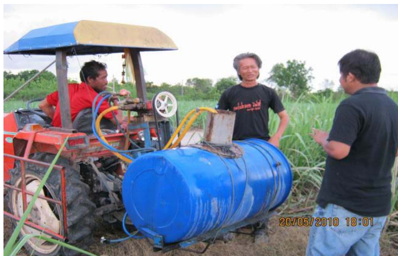
Slim tractor ready for action, 4 spray nozzles at bottom of tank
